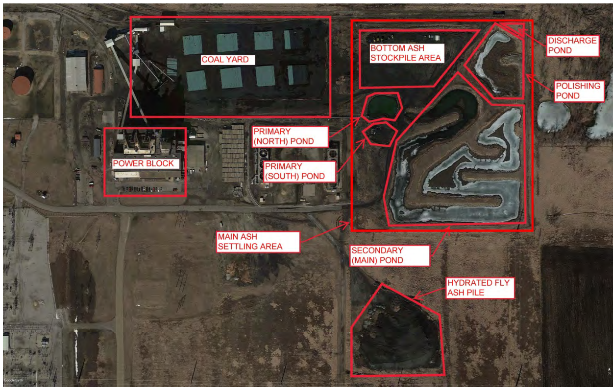
Figure 1 – Current Layout of Sutherland Generating Station
