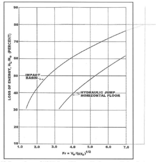
Figure 9.15. Energy Loss of USBR Type VI Impact Basin versus Hydraulic Jump
