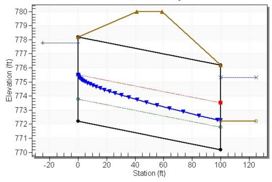
Table 2 - Downstream Channel Rating Curve (Crossing: Haul Road Box Culvert)
