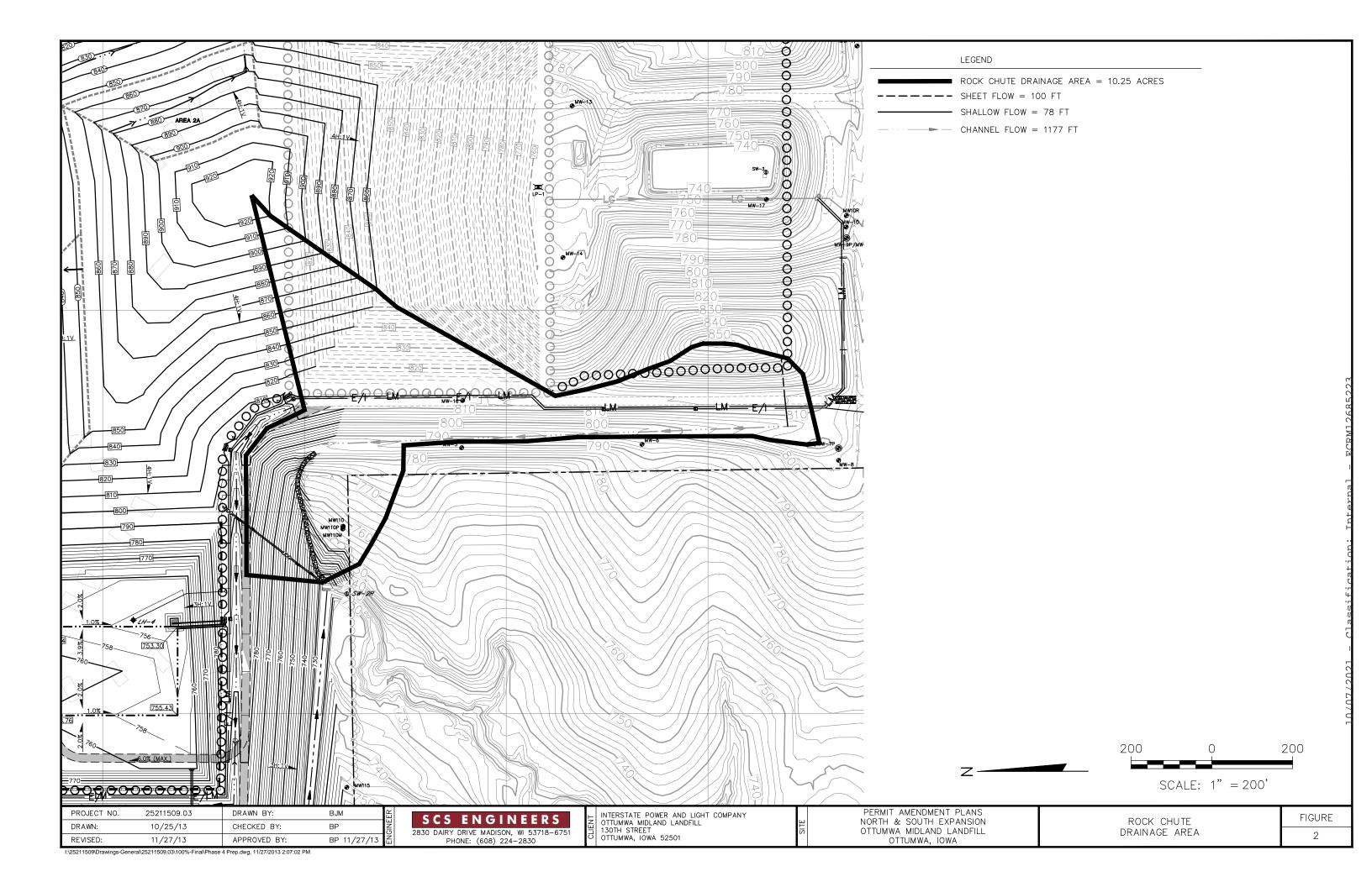
Downslope Flume and Energy Dissipator Sizing
