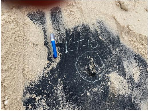
Photograph No. 10 Leak location No. LT-10, a puncture.
