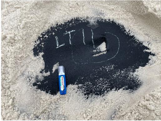
Photograph No. 11 Leak location No. LT-11, a puncture.
