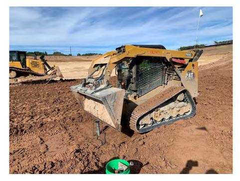
**Photo 42:** Collecting undisturbed clay samples (Shelby tubes) in Modules 10 and 11. (Looking northeast, 09/29/22).
