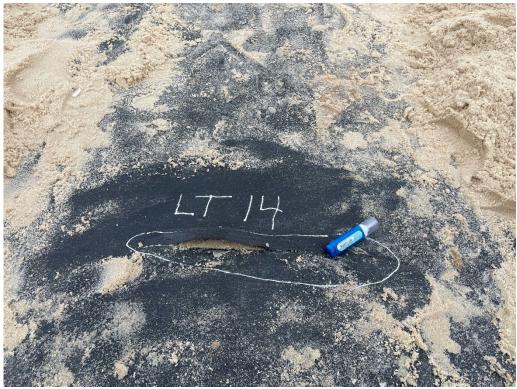
Photograph No. 14 Leak location No. LT-14, equipment damage.
