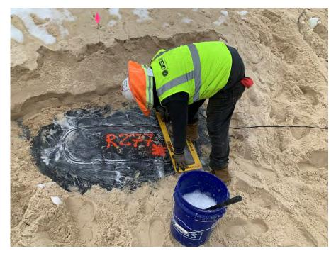
**Photo 112:** Vacuum box testing for the geomembrane repairs. (Looking down, 12/13/22).
