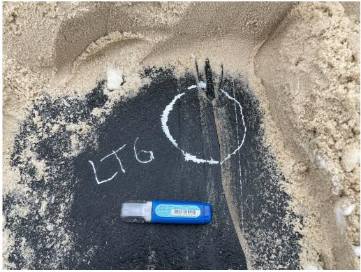
Photograph No. 6 Leak location No. LT-6, a bad extrusion weld.
