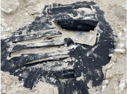
Photograph No. 5 Leak location No. LT-5, equipment damage.
