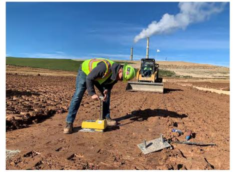
**Photo 41:** SCS conducting moisture/density tests on first foot of clay in Modules 10 and 11 (Looking west, 09/29/22).
