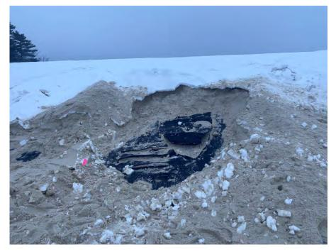
**Photo 106:** Geomembran e damage located by CQM on south slope of Module 10. (Looking south, 12/10/22).
