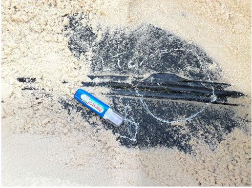
Photograph No. 2 Leak location No. LT-2, a bad extrusion weld.
