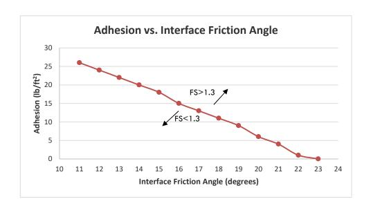
Conclusion: The landfill liner side slope drainage layer was evaluated for static veneer slope stability along its longest slope. Calculations were performed to determine the minimum adhesion necessary for a range of interface friction angles to reach a FS of 1.3 or greater. Each interface friction angle and the coinciding adhesion was graphed in order to easily determine if a material interface is acceptable along the side slope.
