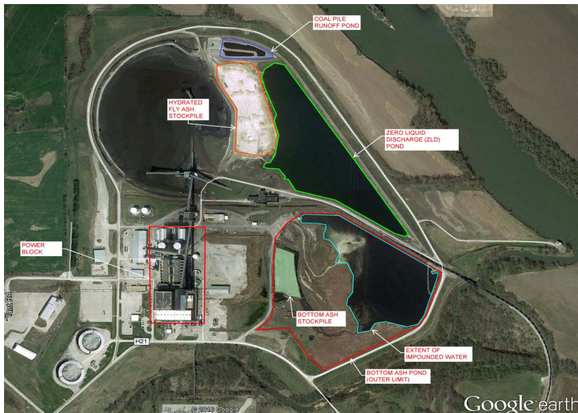
Figure. 1: Overall layout at Ottumwa Generating Station
