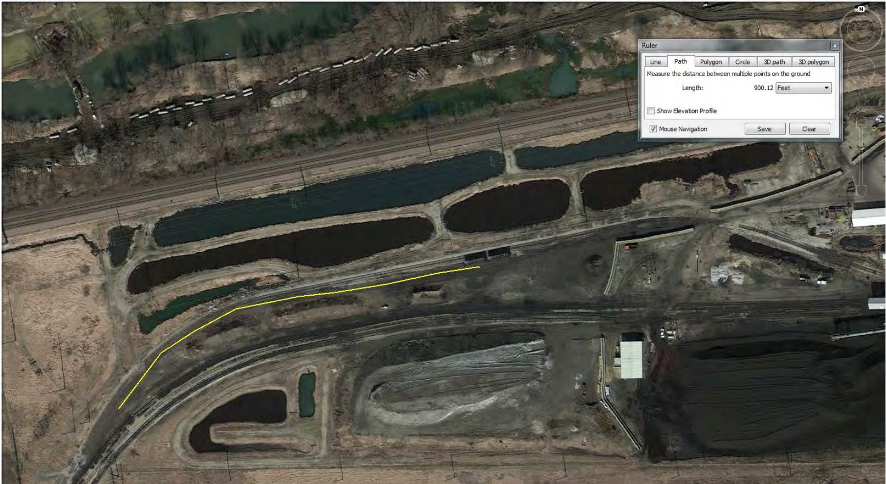
Drainage & Delineation Sketch-Longitudinal limit of low land, north of PCS Bottom Ash Piles - Length 900ft.
