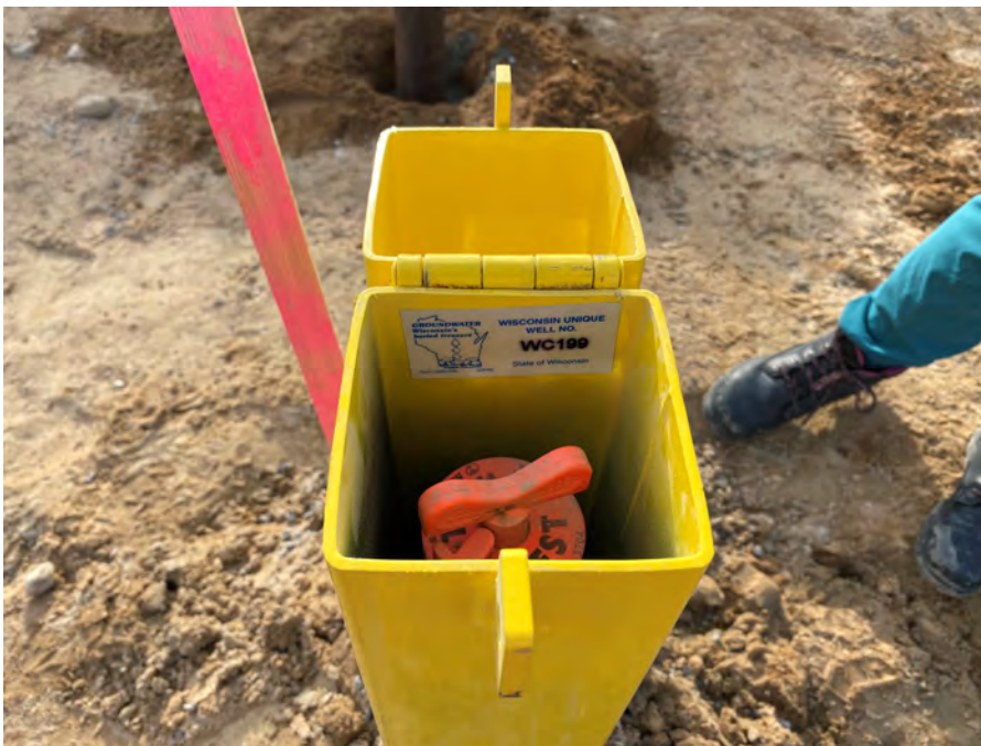
Photo 2: MW-314, view inside protective cover showing WUWN sticker and compression cap. Compression cap to be replaced with a dedicated pump system & integrated cap.
